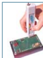
Observe how a ferrite reduces emission
